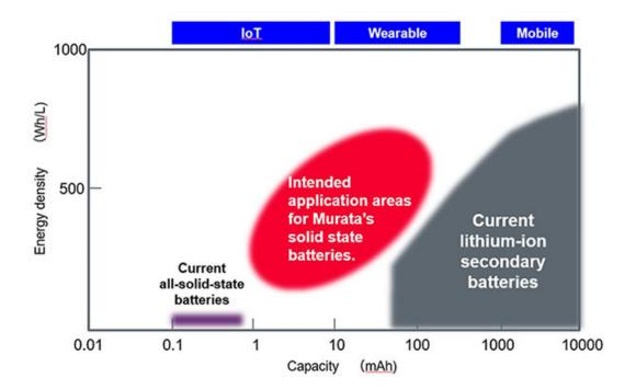
Range of ordinary secondary batteries and target range of solid-state battery
